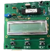
Easy to use 3 button Installer program module with LCD display
