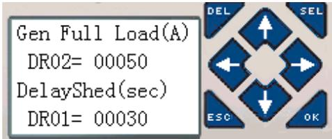
**Generator Full Load DR02-** Adjust to generators maximum amperage output in whole amps.
