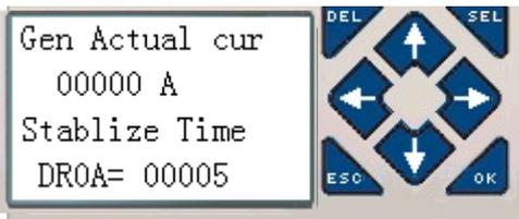
**Actual Real-Time Amps-** Generator amp load as measured by the controllers highest reading on either CT
