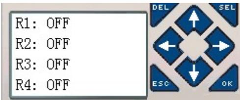
**Real Time State of relays 1-4 (Fixed reading, not adjustable)**
