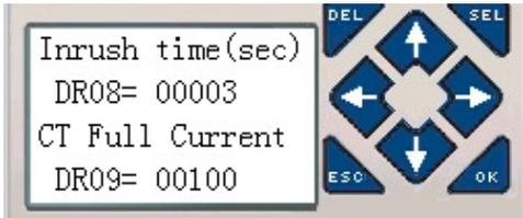
**Generator Inrush Delay DR08-** Adjust allowable In Rush delay time before load shedding will occur
